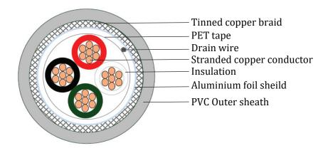
4 core 18AWG (7 strands x 26AWG) braid and foil shielded cable
